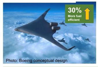
A Blended Wing Body aircraft (above) could be **30% more fuel efficient** than a tube and wing aircraft.
