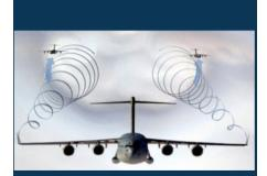
Automated trail, at a safe distance, maintains position in wingtip vortex updraft.
